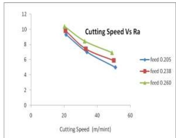
Figure : 6 Double Point cutting tool : First Surface : Cutting speed vs Ra
