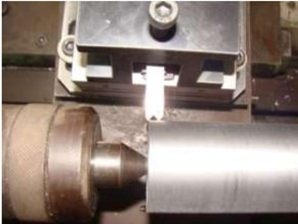
Figure : 1 Double Point Cutting Tool for Turning
