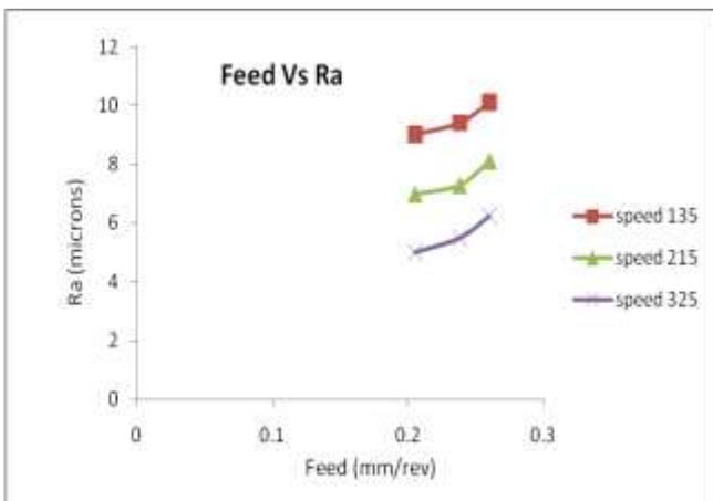
Figure : 9 Double Point cutting tool : Second Surface : Feed vs Ra
