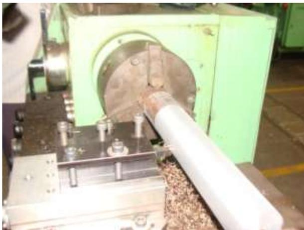
Figure : 2 Double Point Cutting Tool does Turning
