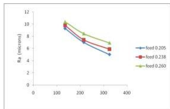
Figure : 4 Double Point Cutting Tool : First Surface : Speed (rpm) Vs Ra( microns)
