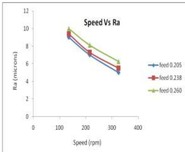
Figure : 5 Double Point Cutting Tool : Second Surface : Speed (rpm) Vs Ra( microns)
