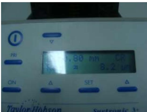
Figure: 3 Taylor – Hobson Surtronic Surface Roughness Measuring Instrument
