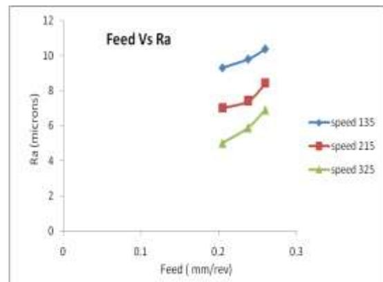
Figure : 8 Double Point cutting tool : First Surface : Feed vs Ra
