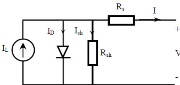
Figure 3.1:- Equivalent circuit of PV solar cell
