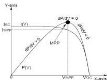
Fig.1. Sign of  $dP/dV$  at different position on the power-voltage characteristic of a PV cell.
