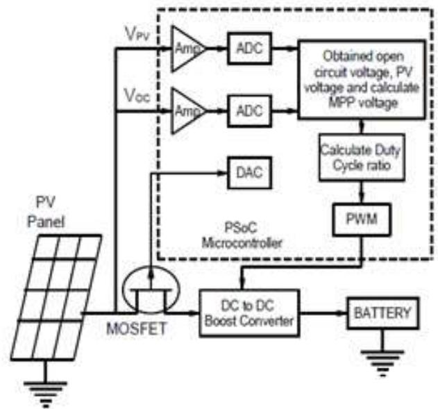
Fig.3. Block diagram of PV System.
