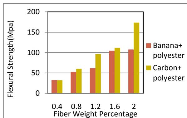
**Fig 10: comparison graph between BANANA fiber and CARBON fiber. (Flexural Strength Vs Fiber weight %)**
