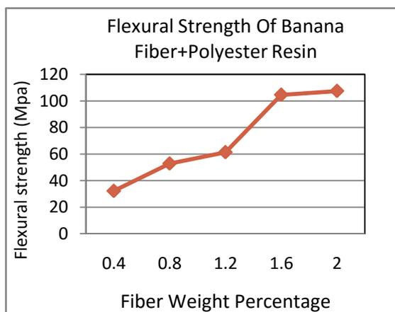
**Fig 5: Flexural strength Vs fiber weight percentage**
