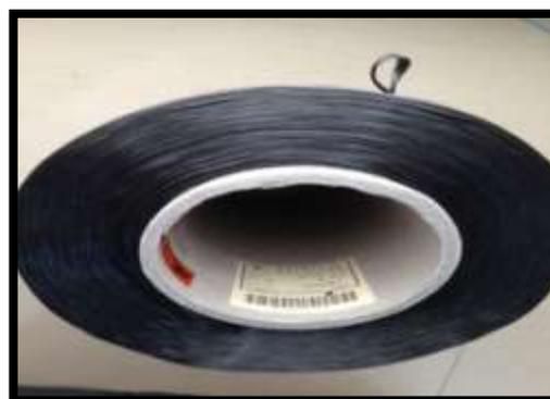
**Fig 3: Bundle of CARBON fiber**
