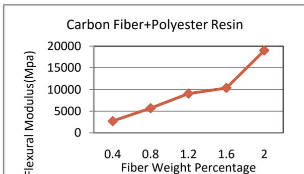
**Fig 8: Flexural modulus Vs fiber weight percentage.**
