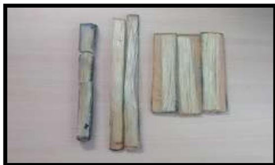
**Fig 2: Fabricated specimens of BANANA fiber**
