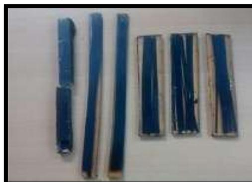
**Fig 4: Fabricated specimens of carbon fiber with polyester resin**
