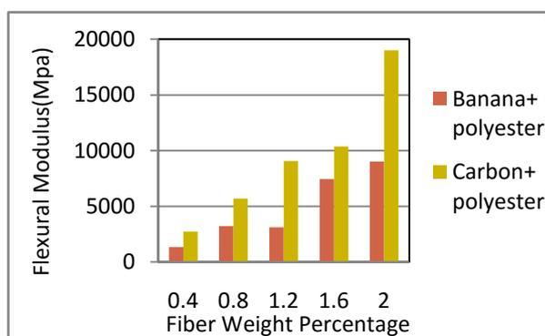
**Fig 9: comparison graph between BANANA fiber and CARBON fiber. (Flexural modulus Vs Fiber weight %)**
