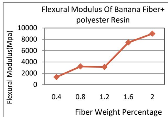
**Fig 6: Flexural modulus Vs fiber weight percentage of BANANA**
