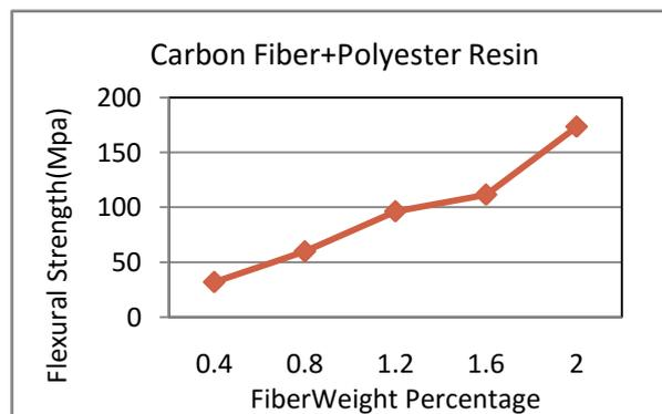
**Fig 7: Flexural strength Vs fiber weight percentages.**
