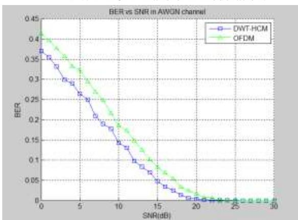
Fig 5: SNR ratio to BER distribution for the OFDM and DWT-HCM Transform modulation
