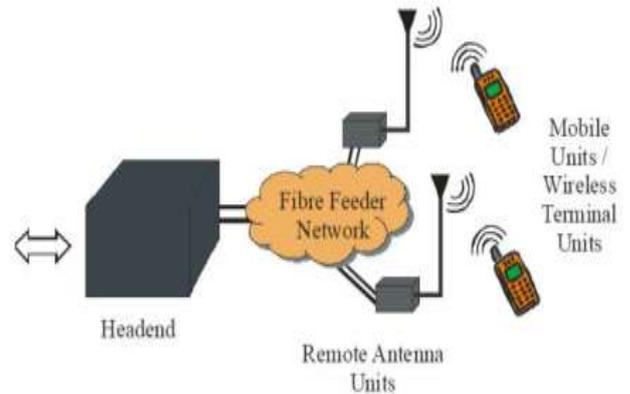
Fig 3: The Radio over Fiber System
