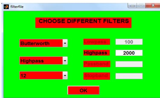
Figure 5.3: Butterworth filter with high pass frequency and 12<sup>th</sup> orders
