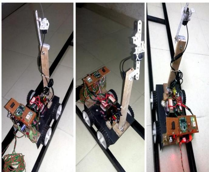
Fig.1.3 Project Model of (Inspection Vehicle unit)
