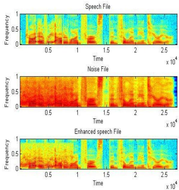
Fig 6. Signal spectrogram with 0db babble noise
