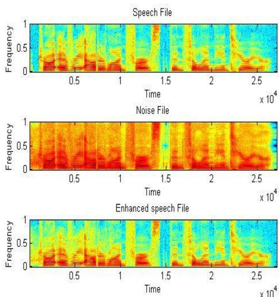
Fig 9 Signal Spectrogramplot at 15 dB babble Noise
