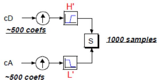
Figure 3 Wavelet Reconstruction: Approximation and Detail coefficient.
