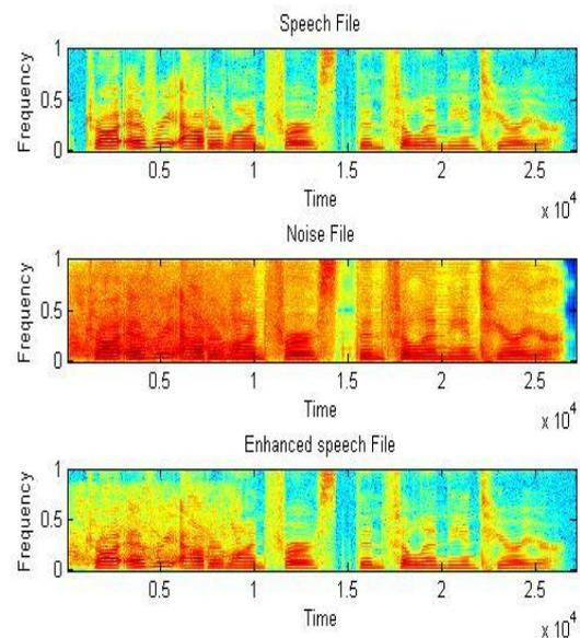
Fig 7. Signal spectrogram at 5db babble noise
