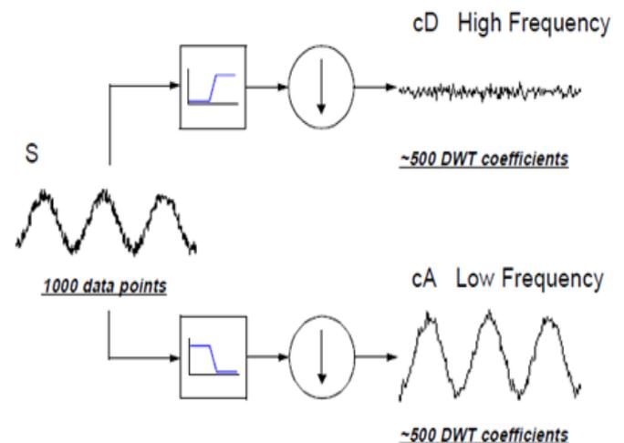
Fig 2. Wavelet Decomposition with filters and Down sampling
