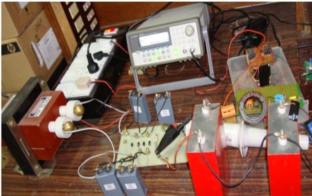
Figure 8: . Set up of 1.5 KV Pulse forming power supply
