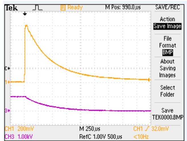
Figure.10. 1.5 KV and 96 A current dumped in Central solenoid coil
