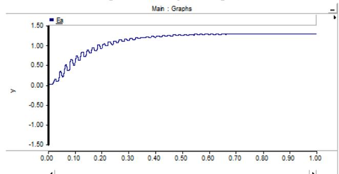
Figure. 4: Voltage wave forms obtained from the voltage multiplier
