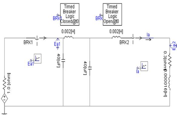
Figure.5: 1KV pulse Discharge with PFN arrangement
