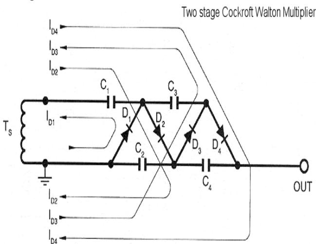
Figure 2 : Ckt of Voltage multiplier
