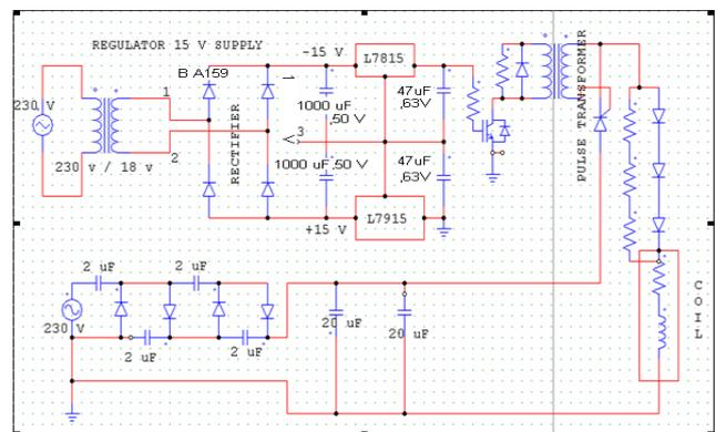
Figure 7 : : Circuit Diagram for 1.5 kv Pulsed Power supply
