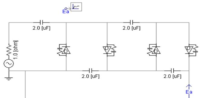
Figure 3: Voltage multiplier circuit to replace the DC source
