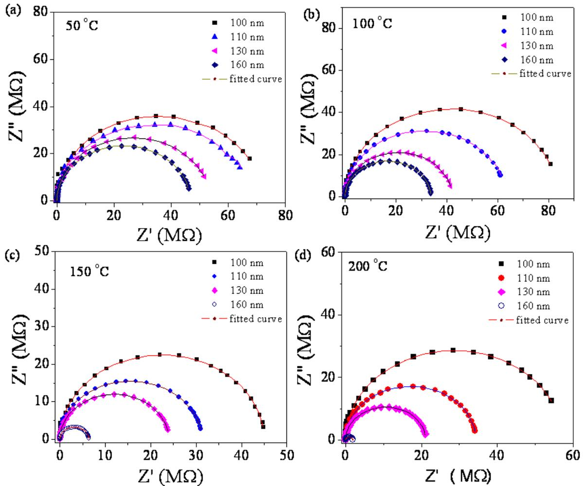
**Fig. 2: The Cole-Cole plots (in log-log scale) of complex impedance spectra of ZnO thin films of various thicknesses as function of temperature (a) 50 °C, (b) 100 °C, (c) 150 °C, and (d) 200 °C**
