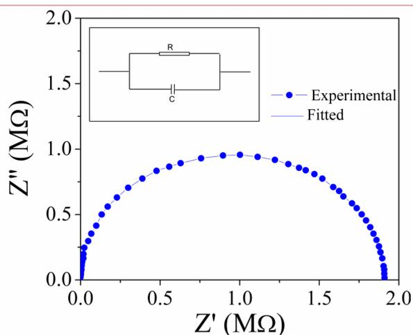
**Fig. 3: A typical impedance spectrum of ZnO thin film with fitted curve showing its semicircular (depressed) nature. Inset shows the proposed equivalent circuit for the experimental data**
