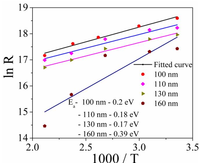
**Fig. 4: Arrhenius plots ( $\ln(R)$  vs  $1000/T$ ) for the ZnO thin films of various thicknesses**
