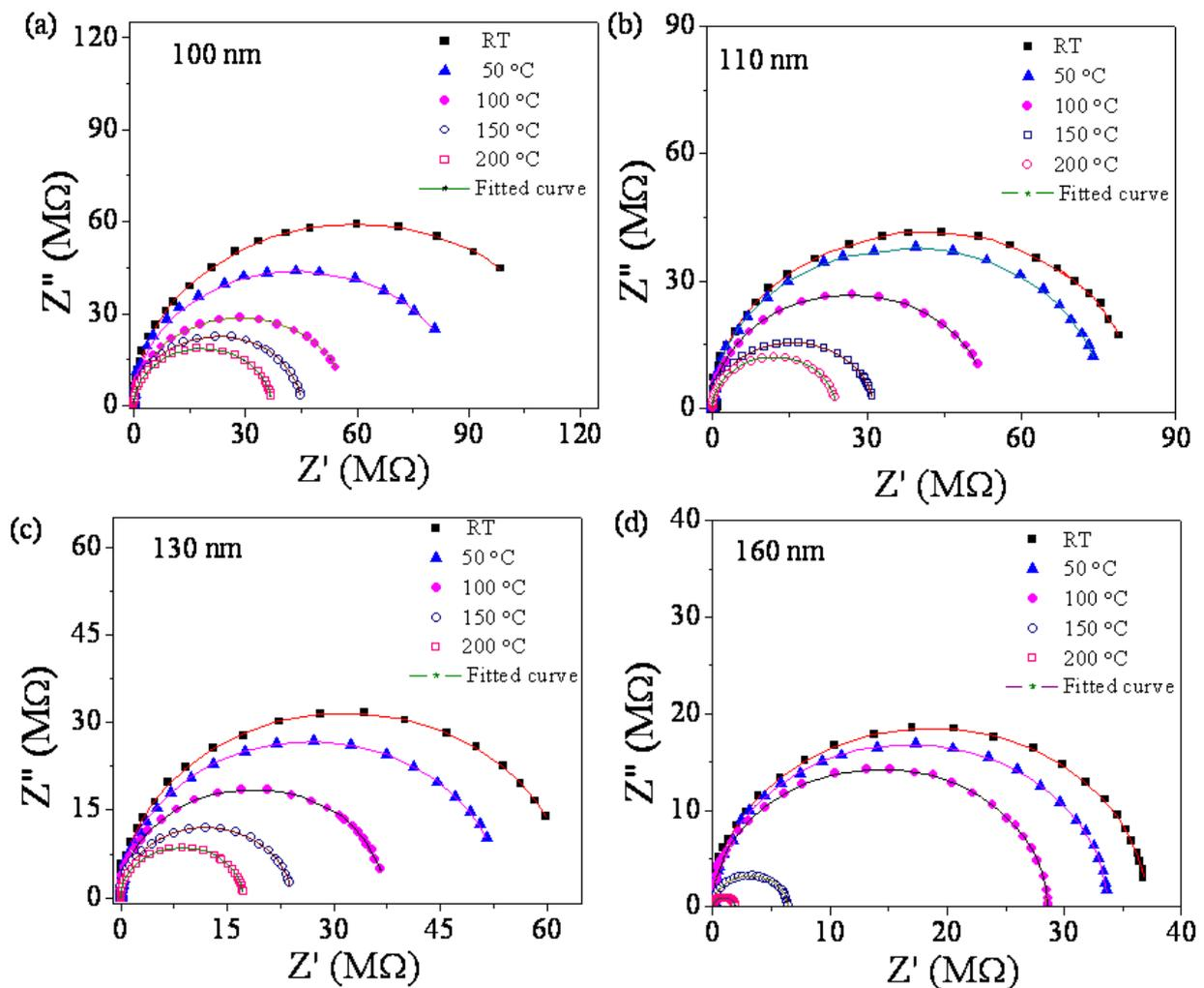
**Fig. 1: The Cole-Cole plots (in log-log scale) of complex impedance spectra of ZnO thin films of (a) 100 nm, (b) 110 nm, (c) 130 nm, and (d) 160 nm thickness at various temperatures in the range RT to 200 °C**
