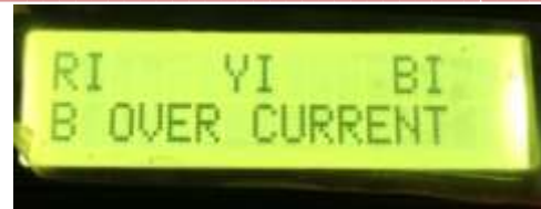
Figure 8: over-current display on LCD
