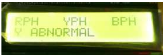
Figure 6: Y phase abnormal display on LCD
