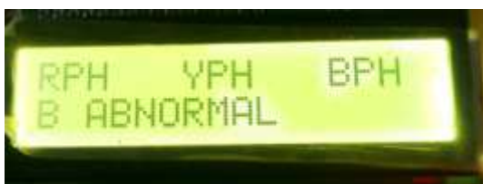
Figure 7: B phase abnormal display on LCD
