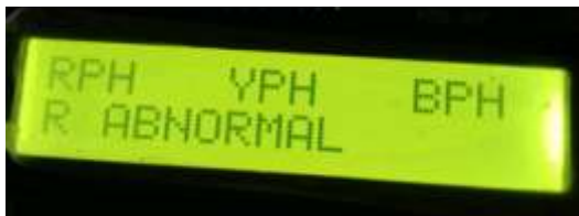
Figure 5: R phase abnormal display on LCD
