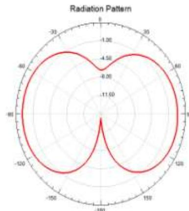
Fig:9: Radiation pattern of antenna with etched inclusion
