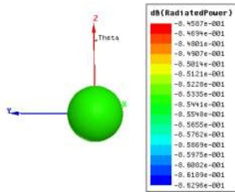
Fig:8 Radiated power for etched AMM inclusion
