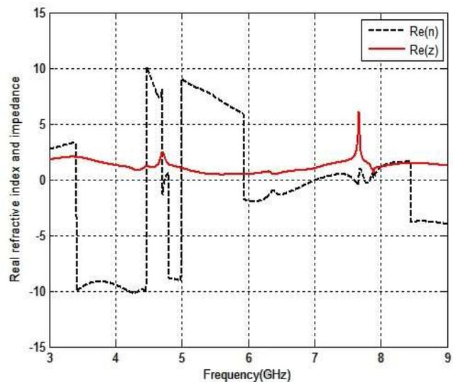
Fig:10: MATLAB plot for negative refractive index for proposed AMM unit
