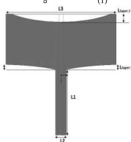
Fig:2 Y-Shaped Antenna without etched AMM Inclusion
