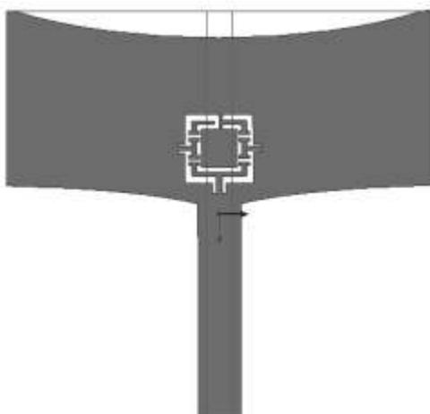
Fig:3 Y-Shaped Antenna with etched AMM Inclusion
