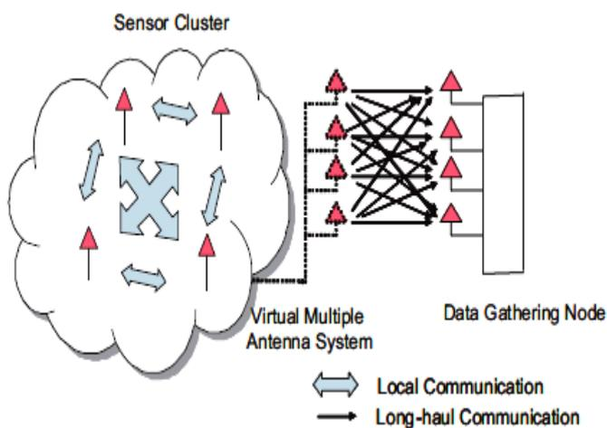
Fig.1 A virtual MIMO communication-based wireless sensor network
