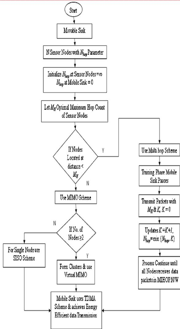
Fig.4. Design Flow for MIHOP Technique
