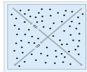
Fig.7 X path cover maximum area in less time
