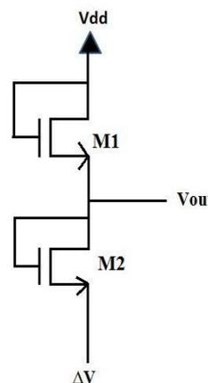
Fig 6 : Basic Pseudo Resistive Divider
