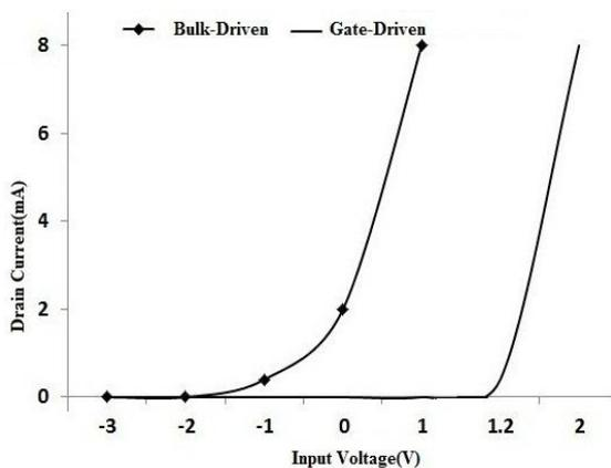
Fig 5: Characteristics plotted for Gate driven and Bulk-driven n channel MOSFET
