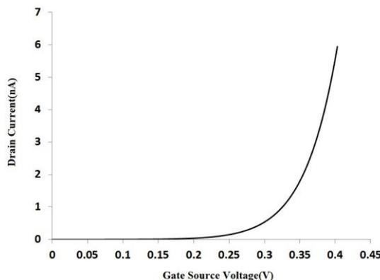
Fig 3:  $I_d - V_{gs}$  characteristics of NMOS for weak inversion operation
