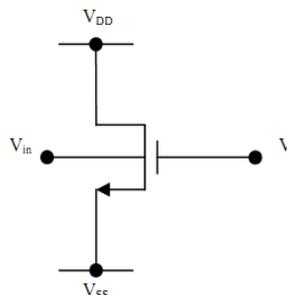
Fig 4: Bulk-driven MOSFET symbol
