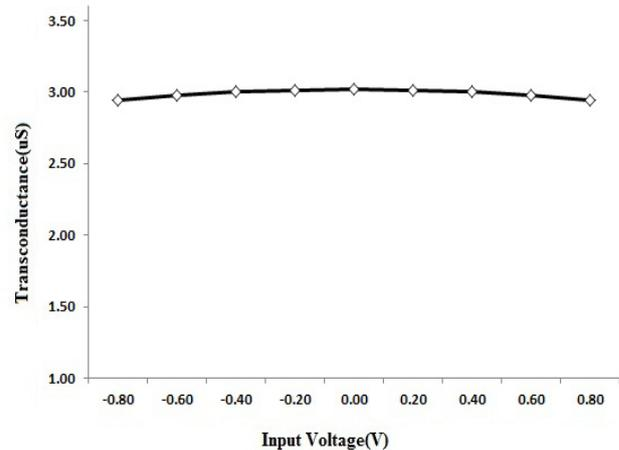
**Fig 11: Transconductance variation (DC) with differential input voltage**
