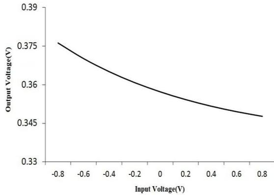
**Fig 9: Output voltage of pseudo resistive divider**
