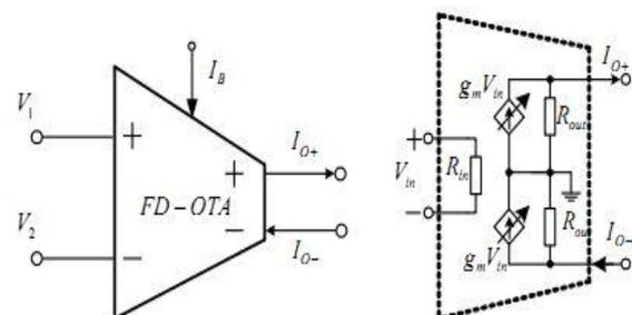
Fig 1: OTA (a) Symbol (b) Equivalent circuit
