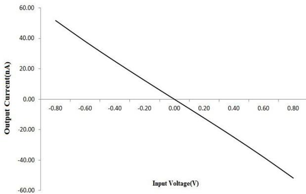
**Fig 12: Output Current variation (DC) with differential input voltage**
