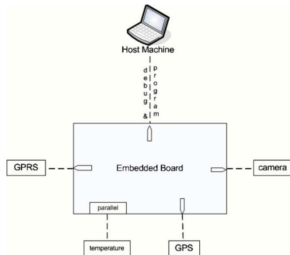
Fig.5. Block diagram of the embedded system with sample devices attached.
