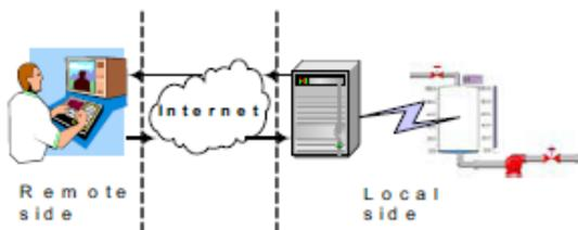
Fig.1.The block diagram of internet-based control system
