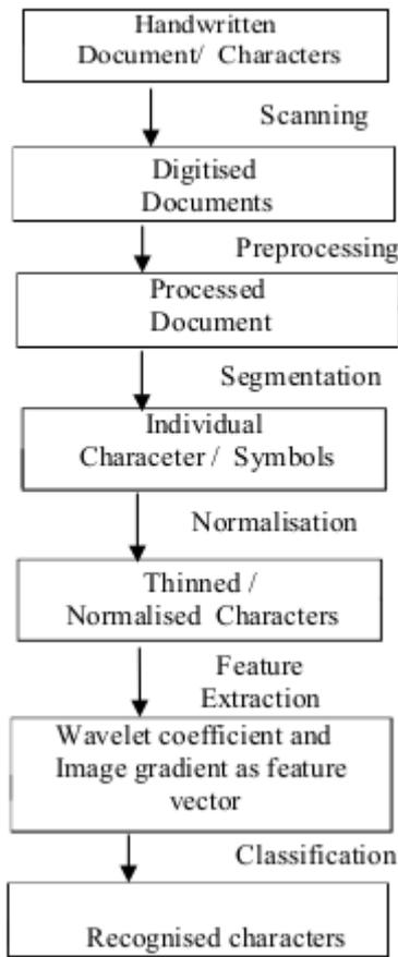
Fig. 2. Block diagram of proposed solution.
