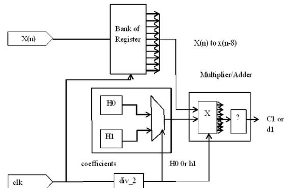
Fig.3 Architecture design of 2D- Discrete Wavelet Transform
