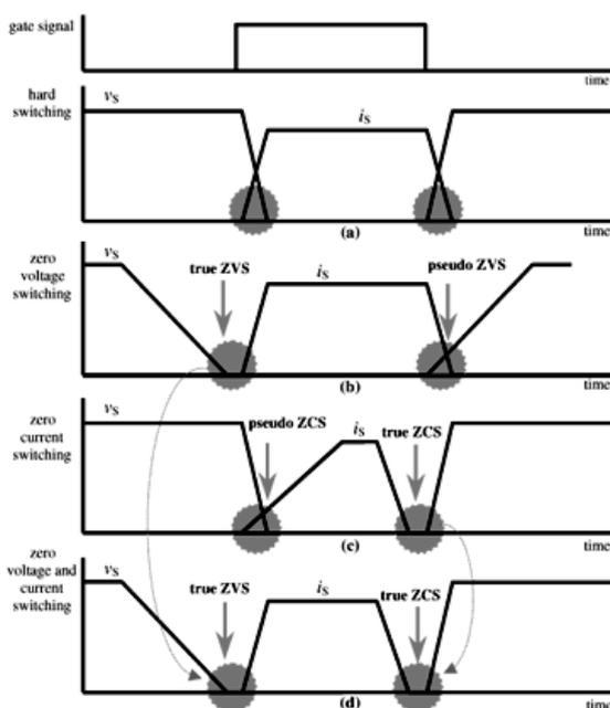
Fig.6. Comparison between switching techniques
