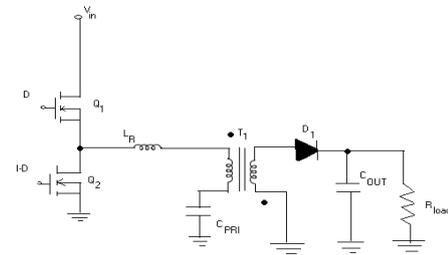
Fig.4. Zero voltage switching converter
