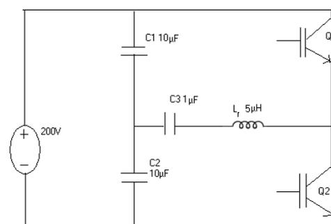
Fig.5. Zero current switching circuit
