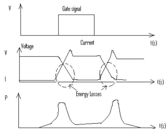
Fig.1 Energy losses during turn on and turn off
