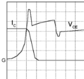
Fig.2. Turn off waveform of IGBT using snubber
