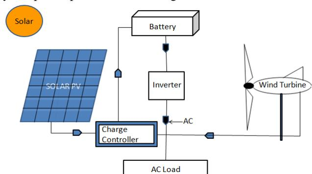
Fig.2. Block diagram of Solar-Wind Hybrid Power System
