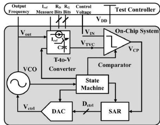
Figure 3 Self-calibrated VCO on-chip system[7]
