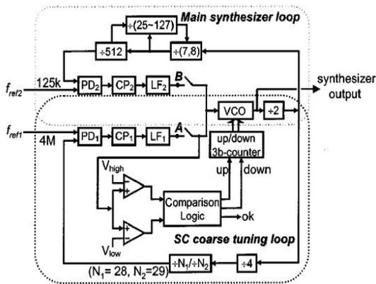
Figure 1. Frequency synthesizer schematic[5]
