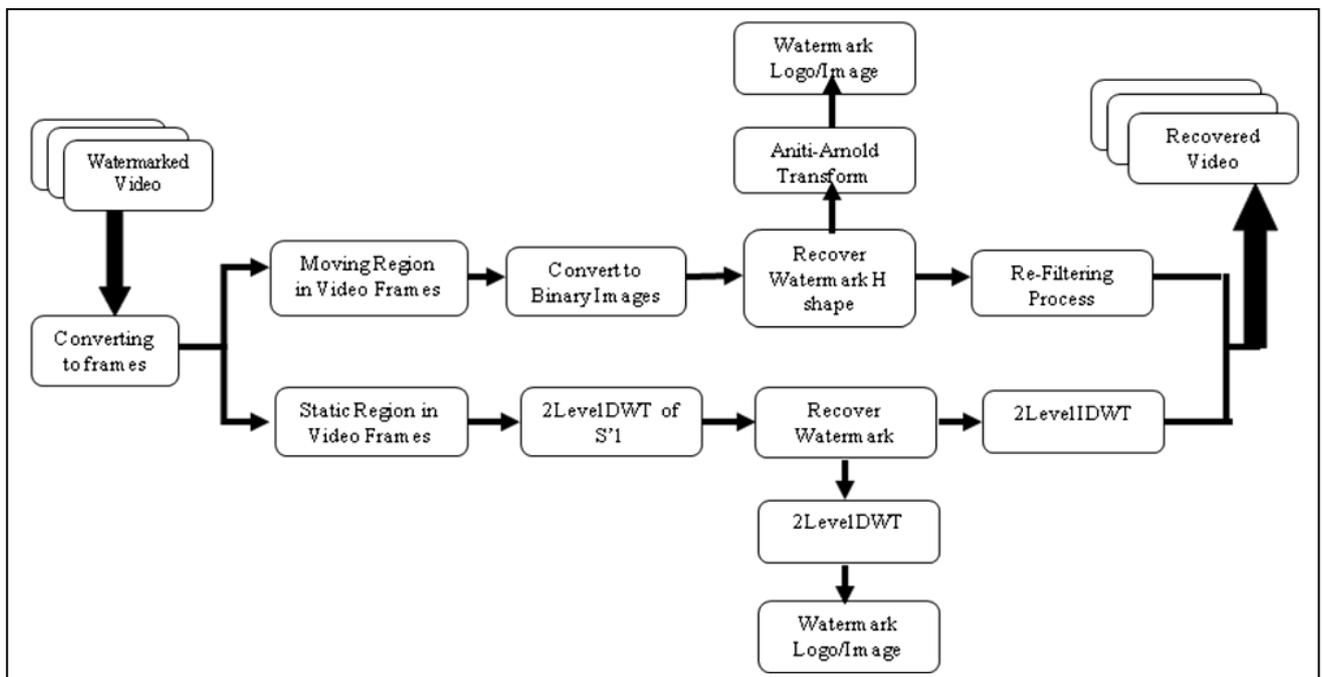
Figure 4. Video Watermark Recovery Process
