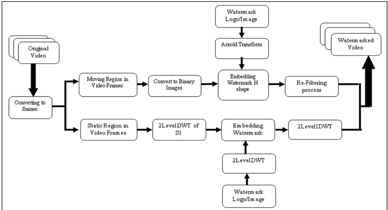
Figure 3. Video Watermarking Embedding Process
