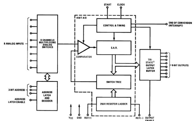
Fig. (1). Block Diagram of ADC
