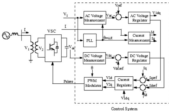
Fig 2 System Model with STATCOM
