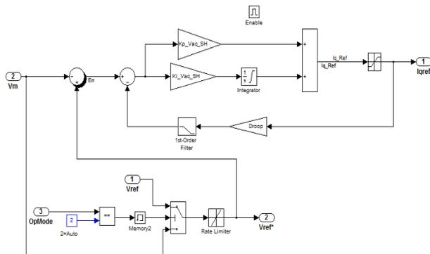
Fig 3 PI Controller connected in STATCOM
