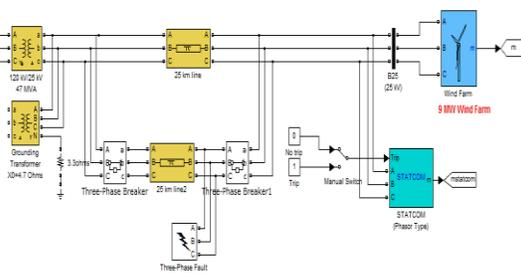
Fig 1 System Model with STATCOM
