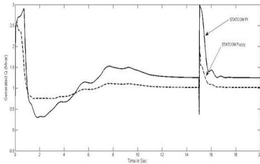
Fig 9 Reactive Power Generated at STATCOM
