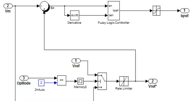
Fig 4 Fuzzy Logic Controller connected in STATCOM
