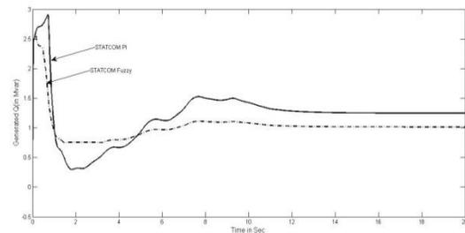
Fig 8 Reactive Power Generated by STATCOM
