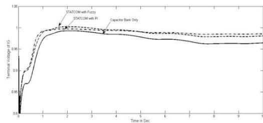
Fig 7 Comparison of the Terminal Voltage of IG under steady state condition
