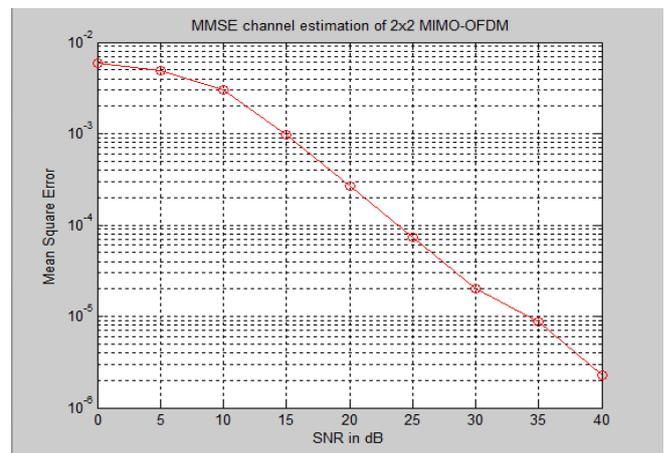
Figure 4 . MSE for MMSE estimation of 2x2 MIMO-OFDM system
