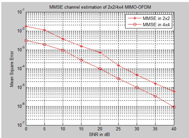
Figure 8 . MSE for MMSE estimation of 2x2 and 4x4 MIMO-OFDM system
