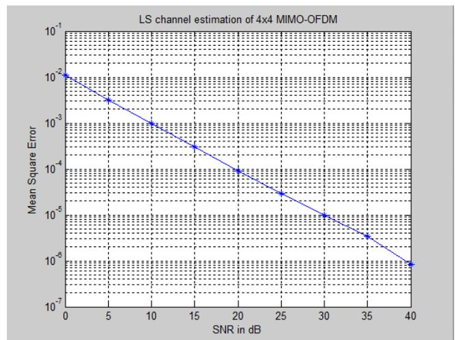
Figure 5. MSE for LS estimation of 4x4 MIMO-OFDM system
