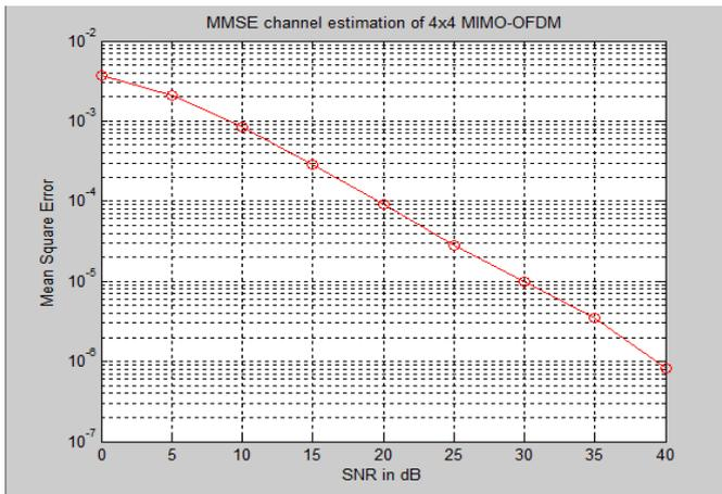
Figure 6 . MSE for MMSE estimation of 4x4 MIMO-OFDM system
