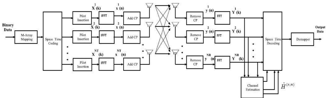
Figure1. MIMO-OFDM System Modelling
