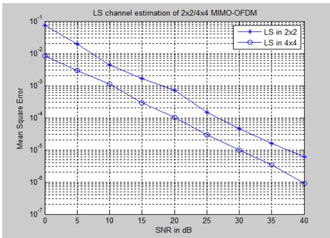
Figure 7 . MSE for LS estimation of 2x2 and 4x4 MIMO-OFDM system
