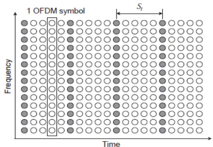
Figure 2. Block Type Pilot
