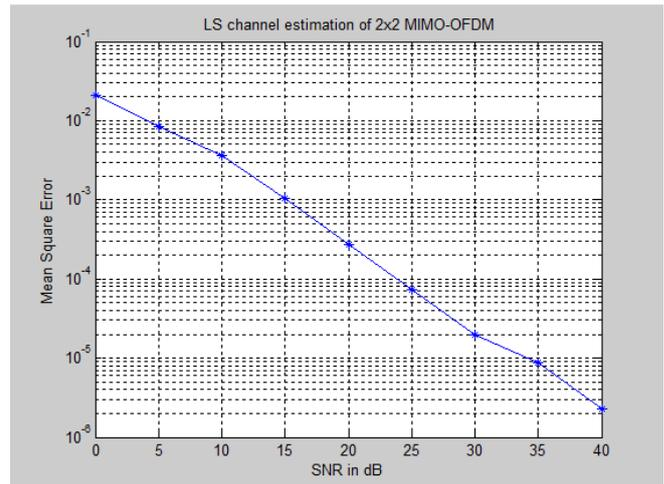
Figure3. MSE for LS estimation of 2x2 MIMO-OFDM system
