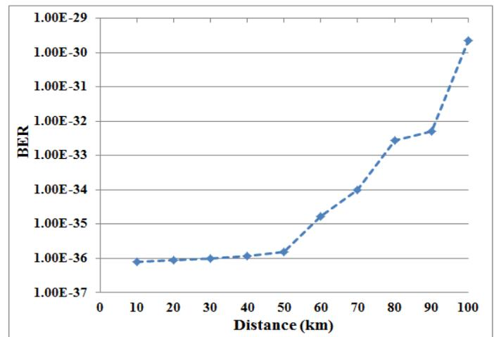
Figure 3: BER versus transmission distance at 2mW input power levels
