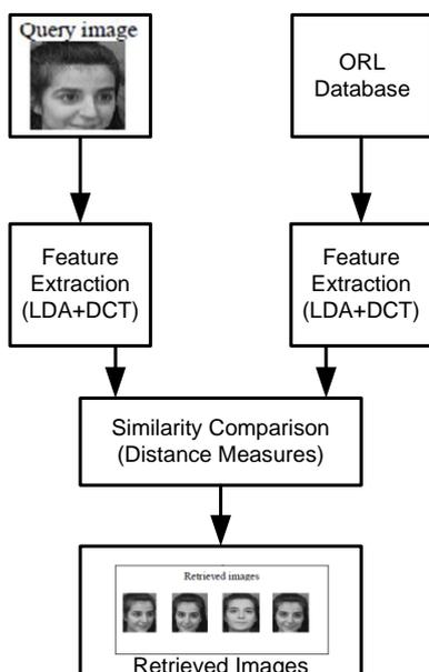
Fig.2 Block Diagram of LDA based Face Recognition
