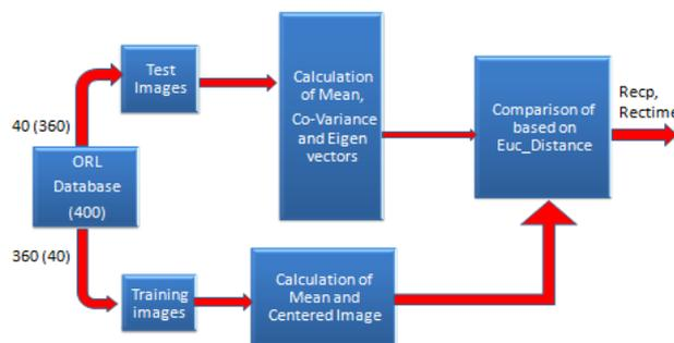
Fig.1 Block Diagram of PCA
