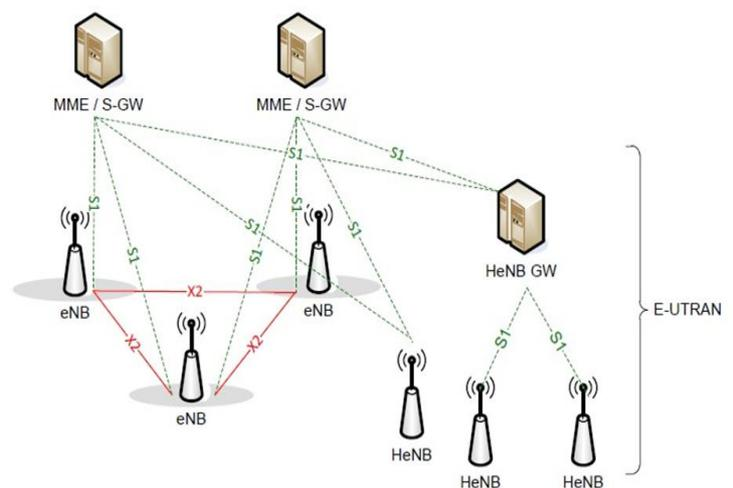
Fig-2 E-UTRAN Architecture with deployed HeNB GW<sup>[2]</sup>
