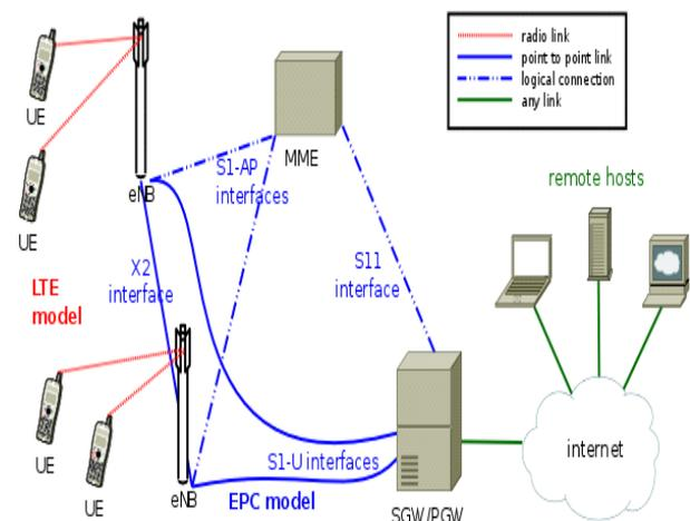
Fig-1 LTE system architecture
