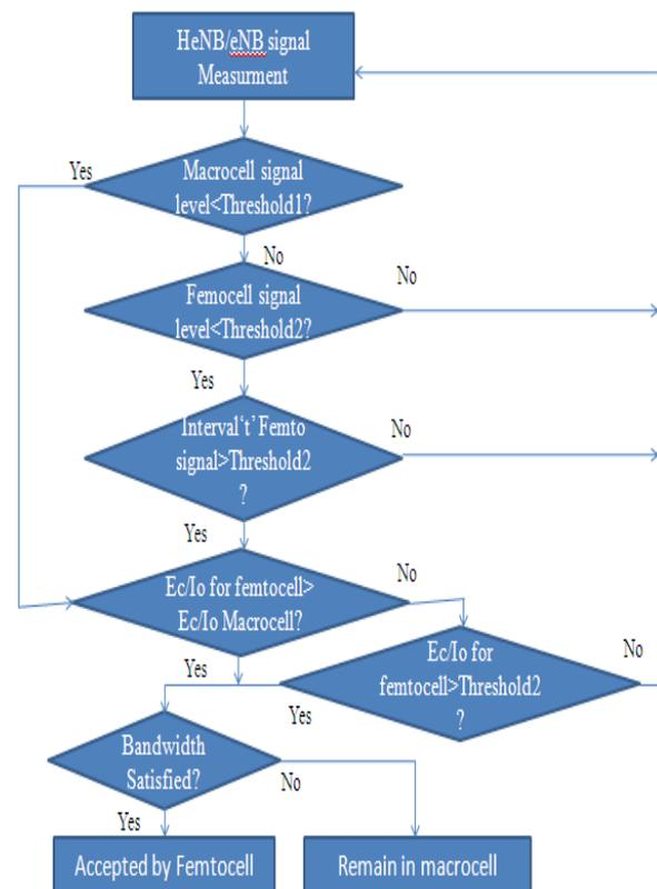
Fig-5 Flowchart of Double Threshold Algorithm [4]
