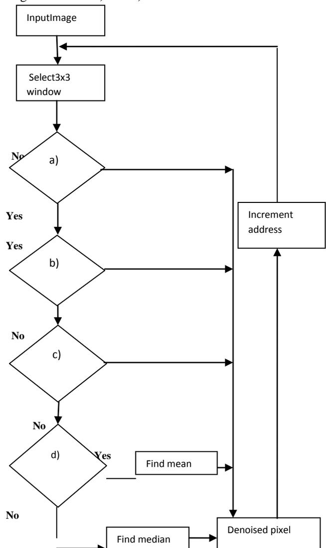
a) Check whether processing pixel is faulty, b) if all window elements are zero, c) if all window elements are 255, d) if window elements are combination of 0 & 255.
