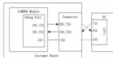
**Figure 7: Debug Port Connection**
