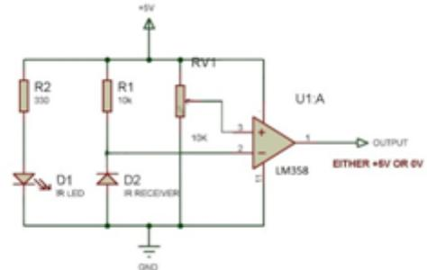
Fig. IR Sensor circuit diagram
