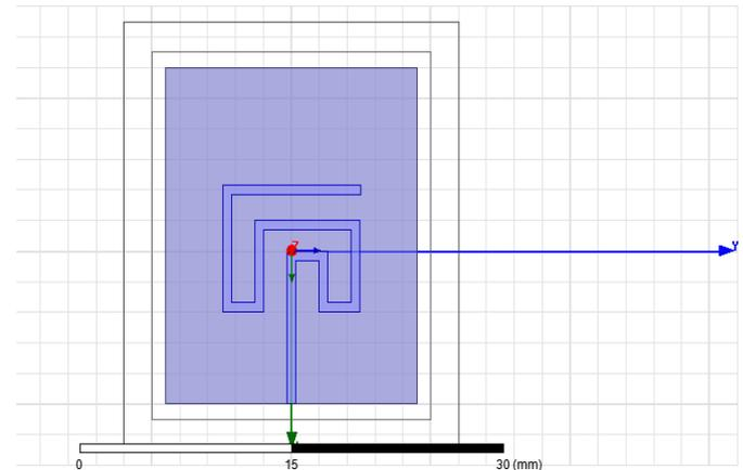
Figure 4 Geometry of antenna optimized with ACO
