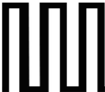
Figure 1 Basic structure of meander line antenna [1]
