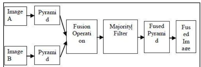
Fig. 4 Laplacian pyramid fusion algorithm
