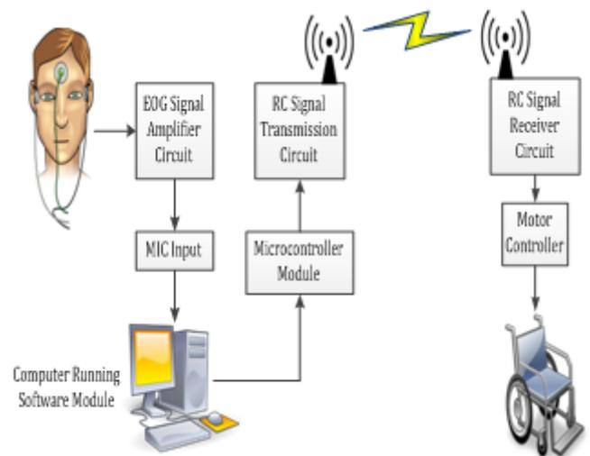
Figure 2: Block diagram of proposed system
