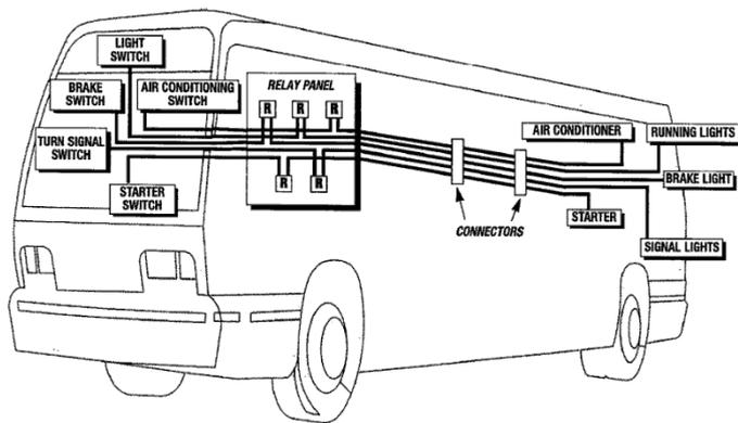
Fig.1. Conventional Vehicle Architecture
