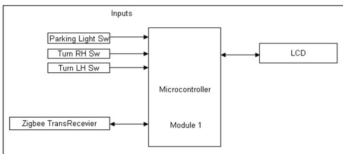
Fig.2. Block Diagram of Node
