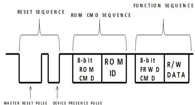
Figure 10. 1-wire command sequence
