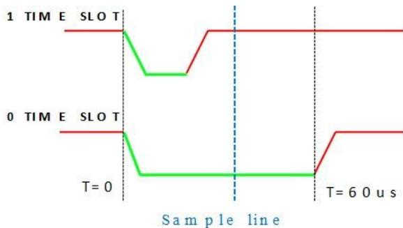
Figure 4. 1 time slot and 0 time slot
