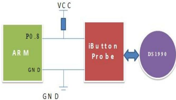
Figure 13. Interfacing between ARM iButton and ARM
