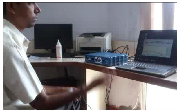
Fig. 3 Biopac MP36 data acquisition system with lead II configuration.
