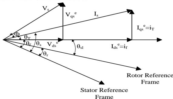
Fig. 2 Phase diagram of vector control
