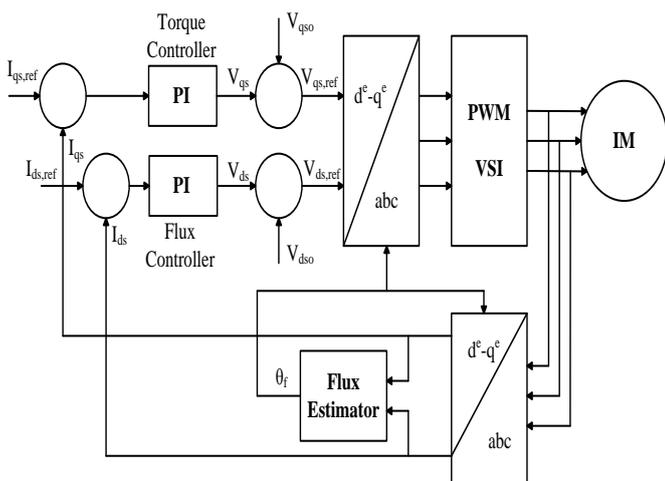
Fig. 3 Block diagram for Indirect Field Oriented Control
