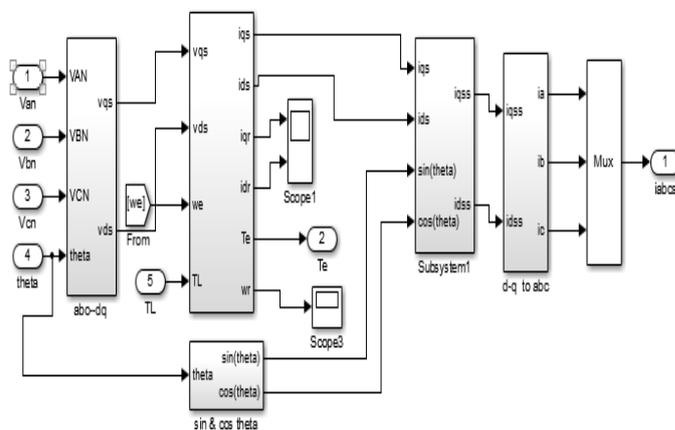
Fig. 7 Simulink Model of Induction Motor
