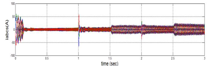
Fig. 13 Phase voltage vao and 3-ph currents of the motor with step changes in load torque
