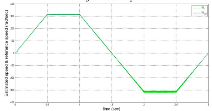
Fig. 14 Four quadrant Estimated speed and reference speed
