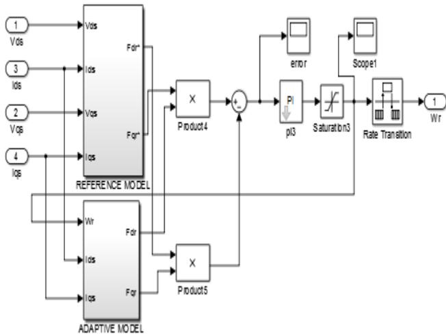
Fig. 8 Simulink Model of Rotor Flux Based MRAS Speed Observer
