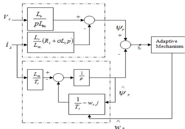
Fig. 6 MRAS based on rotor flux estimation
