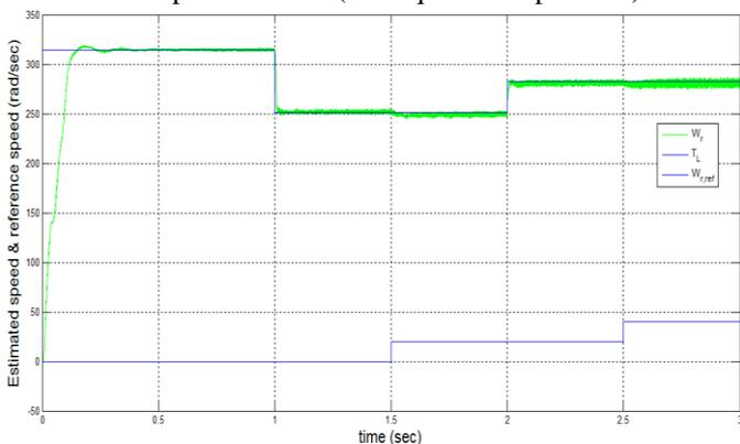
Fig. 10 Estimated and reference speed of the motor with step changes in load torque
