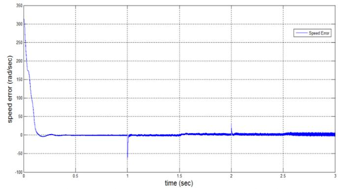
Fig. 11 speed error of the motor for changes in speed and load torque
