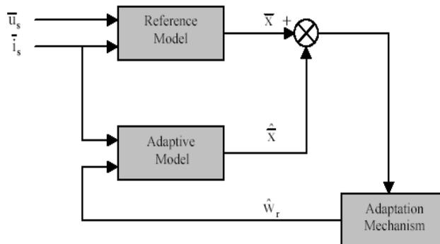
Fig. 5 Generalized model reference adaptive system
