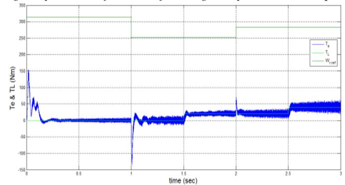
Fig. 12 Generated torque of the motor with step changes in load torque
