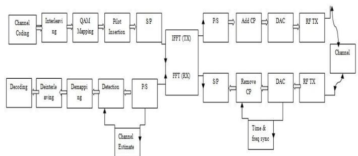
Fig 1. OFDM Baseband Modem
