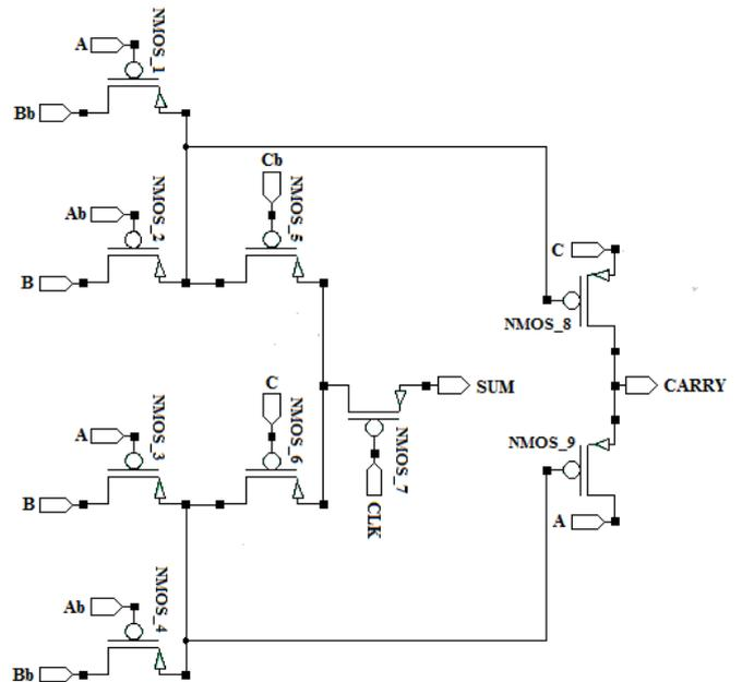
Figure 2. Proposed P-type CPAL Full Adder
