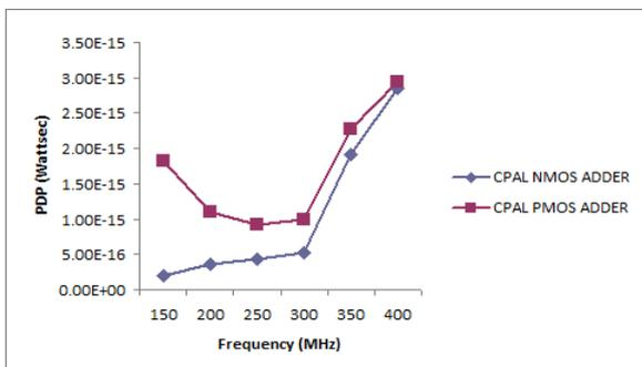
Figure 11. Comparison of PDP for the Adiabatic full adder at different operating frequencies
