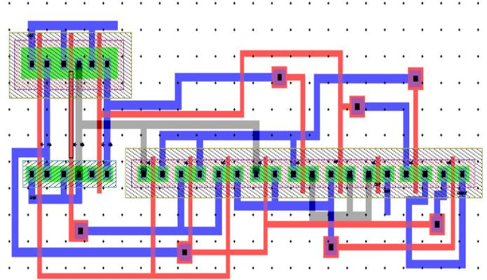
Figure 5. Layout of P-type CPAL Full Adder
