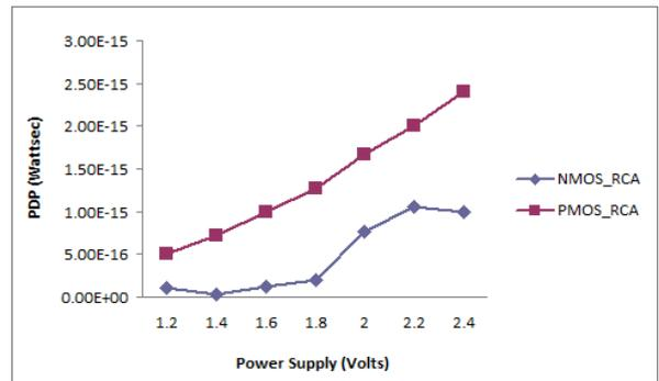
Figure 12. Comparison of PDP for the Adiabatic ripple carry adders at different supply voltages
