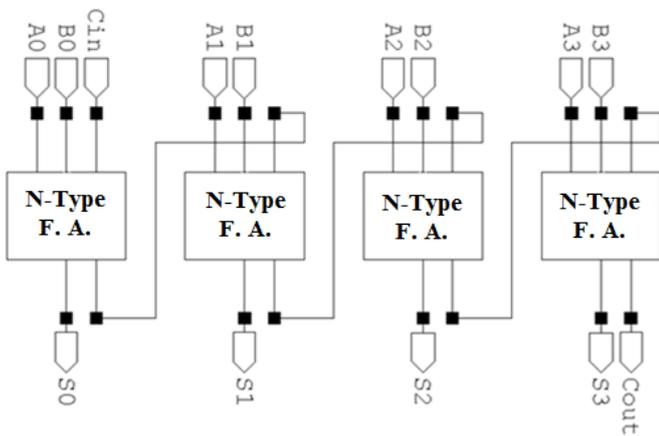
Figure 4. Proposed N-type CPAL Ripple Carry Adder
