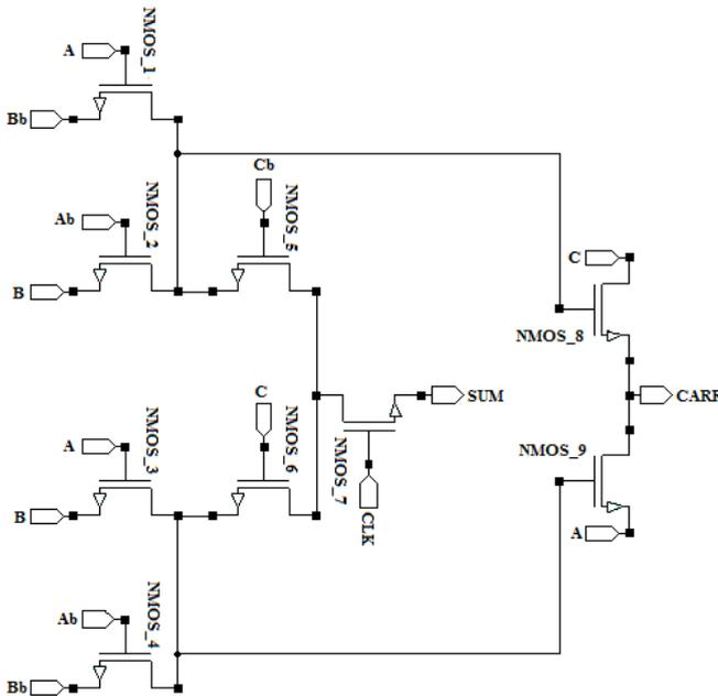
Figure 1. Proposed N-type CPAL Full Adder
