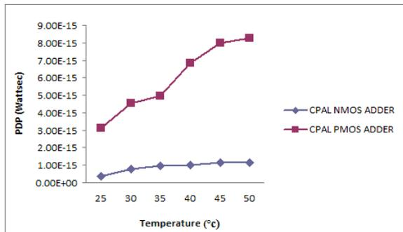
Figure 10. Comparison of PDP for the Adiabatic full adder at different values of temperatures
