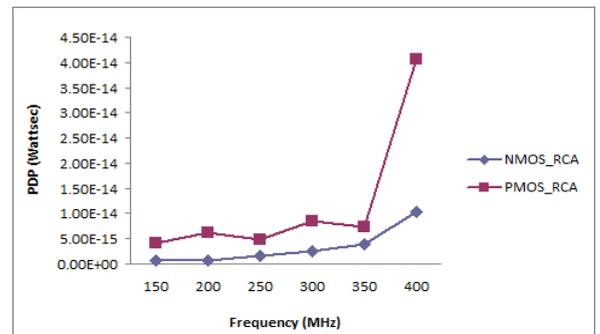
Figure 14. Comparison of PDP for the Adiabatic ripple carry adder at different operating frequencies
