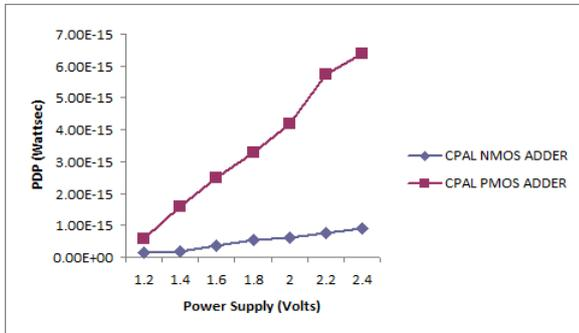
Figure 9. Comparison of PDP for the Adiabatic full adders at different supply voltages
