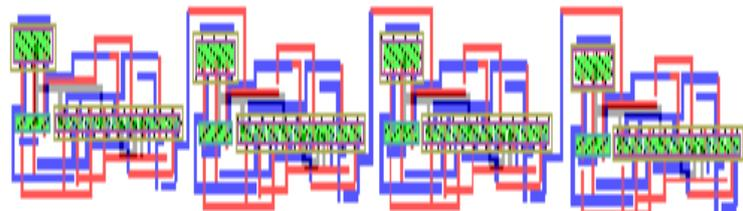
Figure 7. Layout of P-type CPAL Ripple Carry Adder
