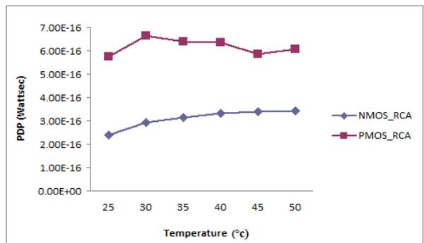
Figure 13. Comparison of PDP for the Adiabatic ripple carry adder at different values of temperatures
