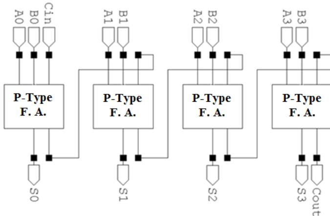
Figure 3. Proposed P-type CPAL Ripple Carry Adder
