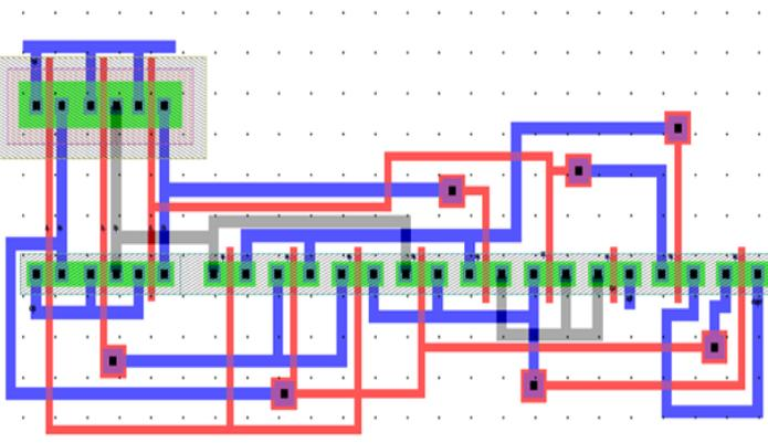
Figure 6. Layout of N-type CPAL Full Adder
