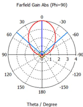
Fig 1.20 Radiation pattern for QWT fed antenna at E-plane,  $\phi=90$ .
