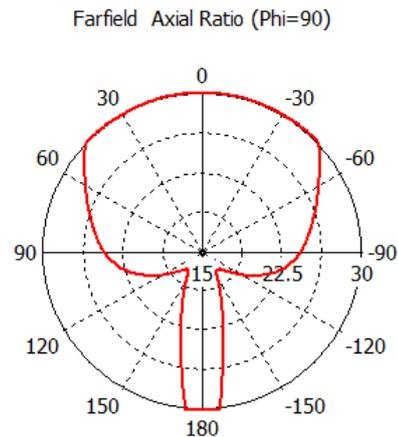
Fig 1.22 Axial Ratio for QWT fed antenna at E-plane,  $\phi=90$ . The Axial Ratio obtained is 30 dB.
