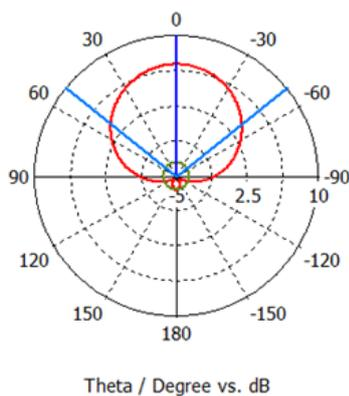
Fig 1.26 Radiation pattern for QWT fed antenna at E-plane,  $\phi=90$ .
