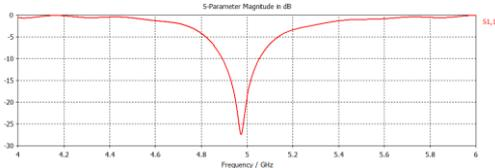
Fig 1.18 Return loss (in dB) for QWT fed antenna at 5 GHz. Return loss for the proposed antenna reaches -27 dB. Bandwidth obtained is 169 MHz.
