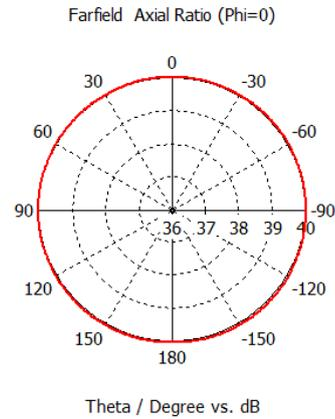
Fig 1.15 Axial Ratio for APMSA fed antenna at H-plane,  $\phi=0$ . The axial ratio obtained is 40 dB.
