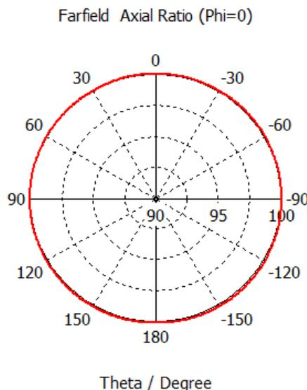
Fig 1.9 Axial Ratio for coaxial fed antenna at H-plane,  $\phi=0$ . The axial ratio obtained is 100 dB. It is perfectly linearly polarized.
