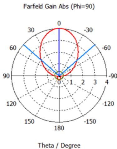
Fig 1.13 Radiation pattern for APMSA fed antenna at E-plane,  $\phi=90$ .
