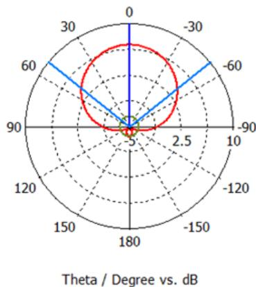
Fig 1.25 Radiation pattern for QWT fed antenna at H-plane,  $\phi=0$ .
