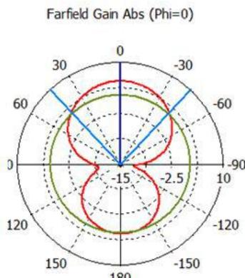
Fig 1.14 Radiation pattern for APMSA fed antenna at H-plane,  $\phi=0$ . The main lobe magnitude (gain) is found to be 5.278 dB.
