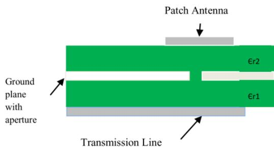
Fig 1.3 Aperture coupled feed
