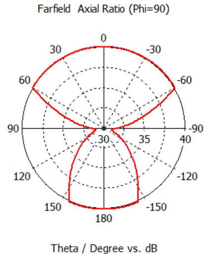
Fig 1.16 Axial Ratio for APMSA fed antenna at E-plane,  $\phi=90$ . The axial ratio obtained is 40 dB.
