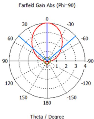
Fig 1.8 Radiation pattern for coaxial fed antenna at E-plane,  $\phi=90$ .
