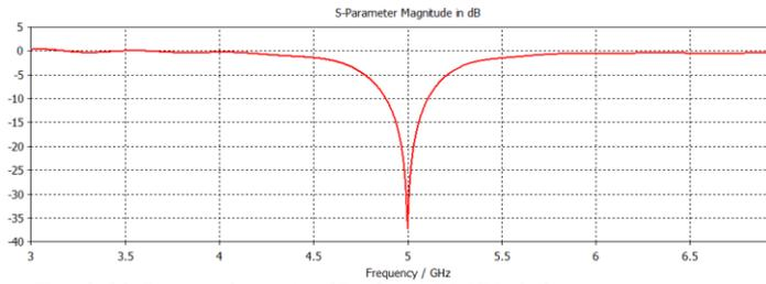
Fig 1.12 Return loss (in dB) for APMSA fed antenna at 5GHz. Return loss for the proposed antenna reaches -37.318 dB, it has the bandwidth of 248 MHz.
