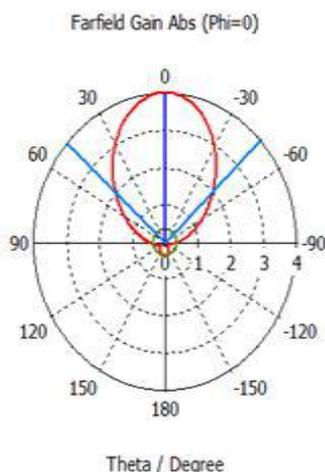
Fig 1.7 Radiation pattern for coaxial fed antenna at H-plane,  $\phi=0$ . The main lobe magnitude (gain) is found to be 3.998 dB.
