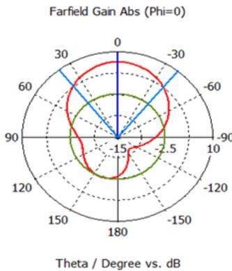
Fig 1.19 Radiation pattern for QWT fed antenna at H-plane,  $\phi=0$ .
