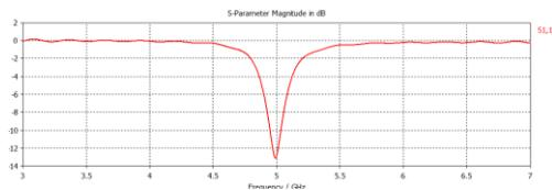
Fig 1.6 Return loss (in dB) for coaxial fed antenna at 5 GHz. Return loss for the proposed antenna reaches  $-13.113$  dB, it has the bandwidth of 98 MHz.
