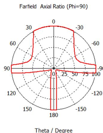
Fig 1.10 Axial Ratio for coaxial fed antenna at E-plane,  $\phi=90$ . The axial ratio obtained is 100 dB. It is perfectly linearly polarized.
