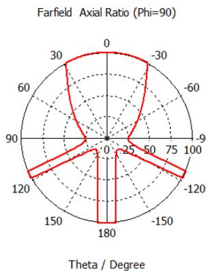
Fig 1.28 Axial Ratio for QWT fed antenna at E-plane,  $\phi=90$ . The Axial Ratio obtained is 120 dB.
