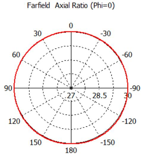
Fig 1.21 Axial Ratio for QWT fed antenna at H-plane,  $\phi=0$ . The Axial Ratio obtained is 30 dB.
