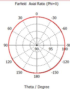
Fig 1.27 Axial Ratio for QWT fed antenna at H-plane,  $\phi=0$ . The Axial Ratio obtained is 100 dB. It is perfectly linearly polarized.
