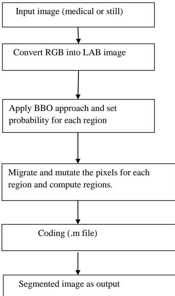
Fig. 2:-Flowchart of purposed work
