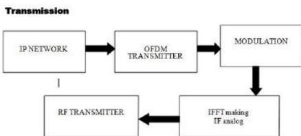
An OFDM transmitter accepts data from an IP network, converting and encoding prior to modulation .An IFFT(inverse fast Fourier transform) transforms the OFDM signal into an IF signal, which is sent to RF transmitter. With orthogonal sub-carriers, the receiver can separate and process each sub-carrier without interference from other sub-carriers. OFDM provides better link and communication quality. It is more impervious to fading and multi-path delays than other transmission techniques.
