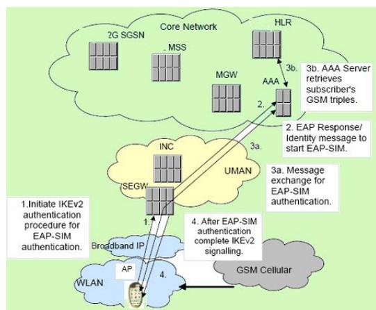
Fig. 5 UMA Authentication Procedure
