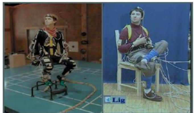
Fig- 4: Mechanical Mocap System
