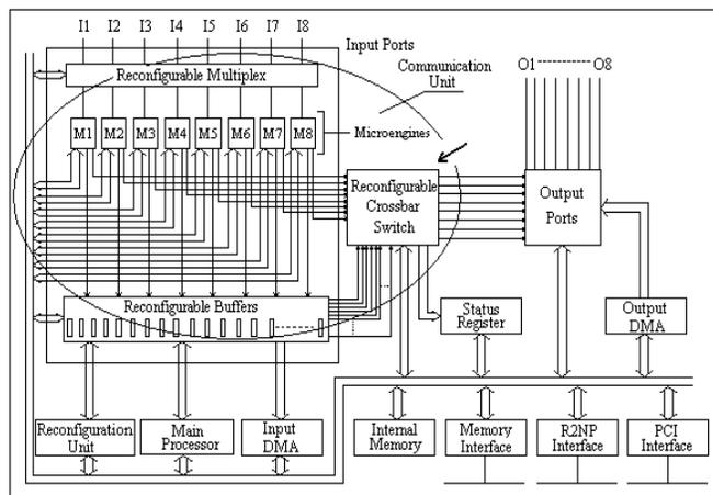
Fig.5 R2NP (Reconfigurable RISC Network Processor) architecture
