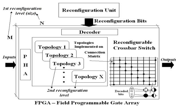
Fig.1 FPGA –Reconfigurable Crossbar Switch.
