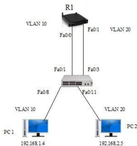
Fig 2 Router and PC Communication.
