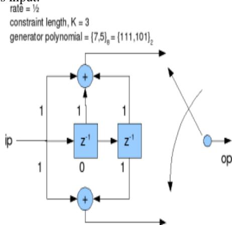
Figure 1: Convolutional code with Rate 1/2, K=3, Generator Polynomial [7, 5] octal
