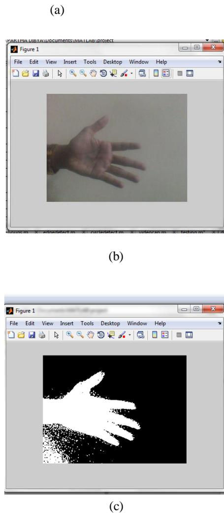
Figure 2. (a) The background image, (b) the background image with foreground (hand), (c) the background subtracted image
