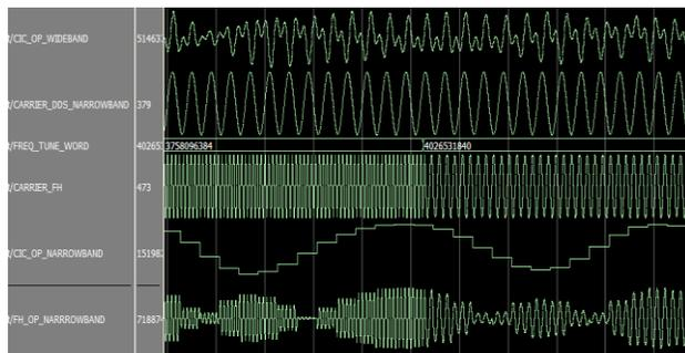
Figure 10: Functional Simulation Results for Narrowband Channelizer and FH
