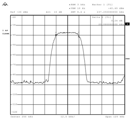
Figure15: Extracted 25 KHz Narrowband Channel
