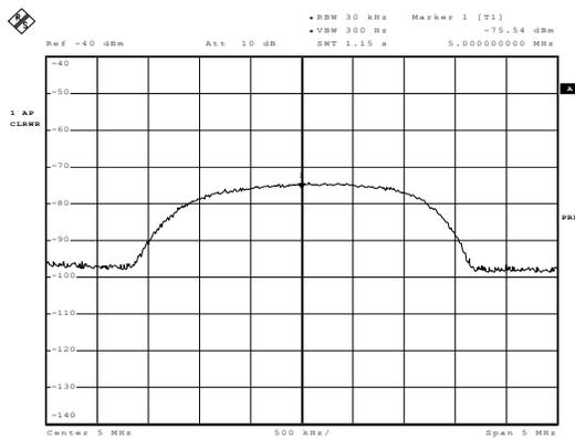
Figure14: Extracted 2 MHz Wideband Channel
