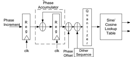
Figure 5: Architecture of DDS in FPGA
