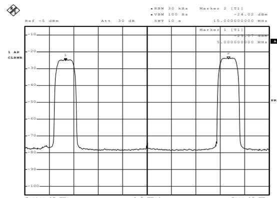
Figure 12: Multichannel Signal from VSG
