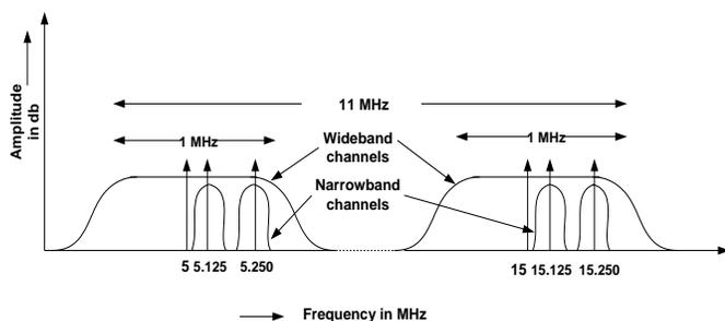
Figure 2: Frequency plan
