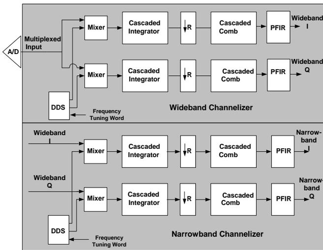
Figure 4: Wideband and Narrowband Channelizer Architecture using DDC Technique
