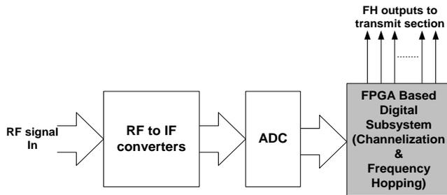
Figure 1: Basic block diagram of proposed SATCOM System
