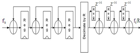
Figure 6: CIC Decimator Filter Architecture
