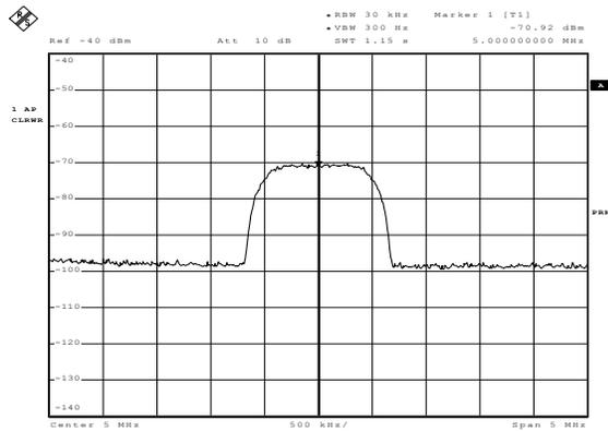
Figure13: Extracted 1 MHz Wideband Channel
