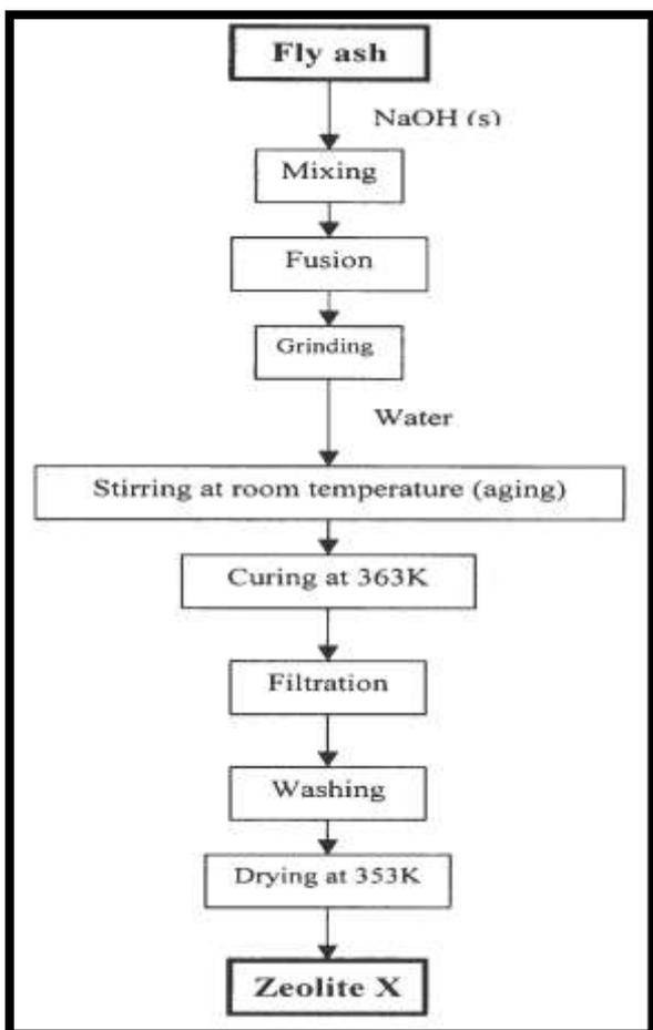
Fig b: Process flow diagram for synthesis of zeolite X-type from fly ash
