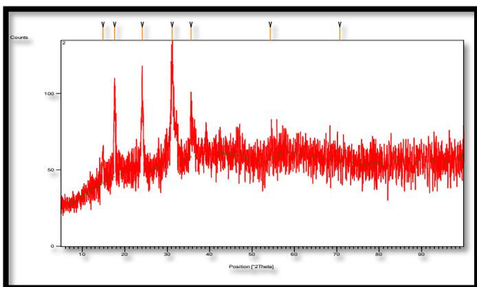
Figure 2 a: X-ray diffraction of zeolite
