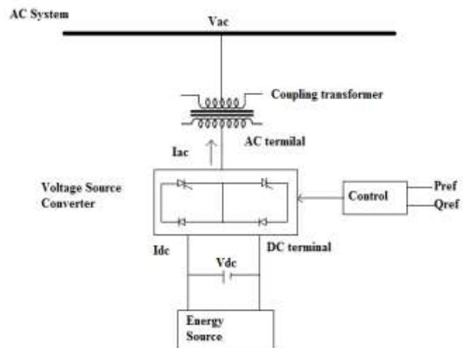
Figure 1: Functional block diagram of STATCOM
