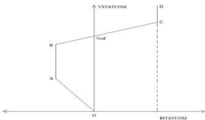
Fig 2: V-I Characteristics of STATCOM
