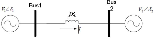
Figure 3 Power transmission system
