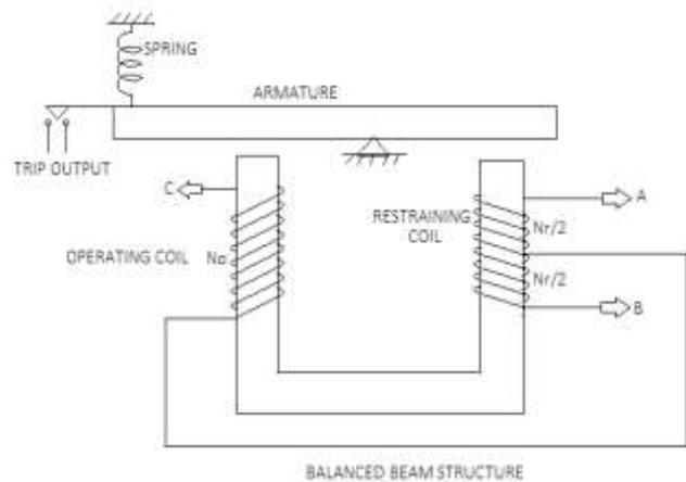
Figure 4. Balanced beam structure
