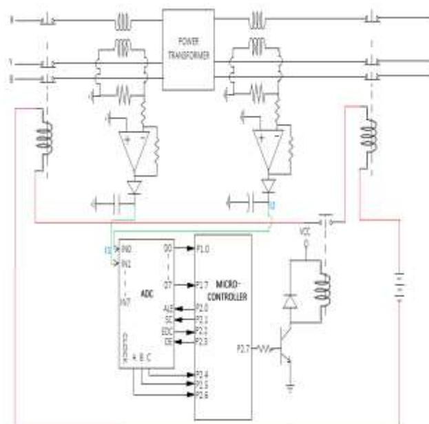
Figure 7. Interfacing with microcontroller
