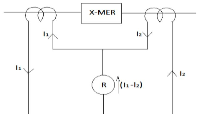
Figure 1. Simple differential protection
