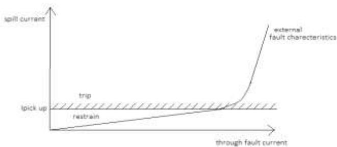
Figure 2. Characteristics of simple differential relay
