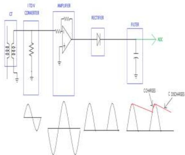
Figure 6. Circuit diagram showing conversion of primary current to the digital form compatible with microcontroller
