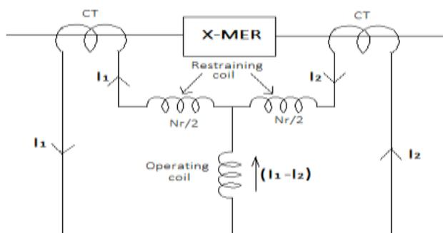
Figure 3. Percentage/biased differential relay
