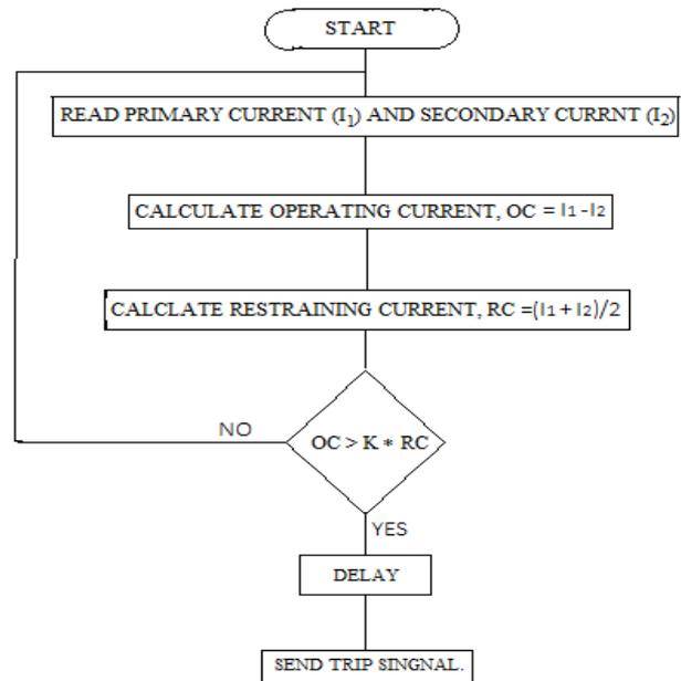
Figure 8. Flow chart for percent differential protection
