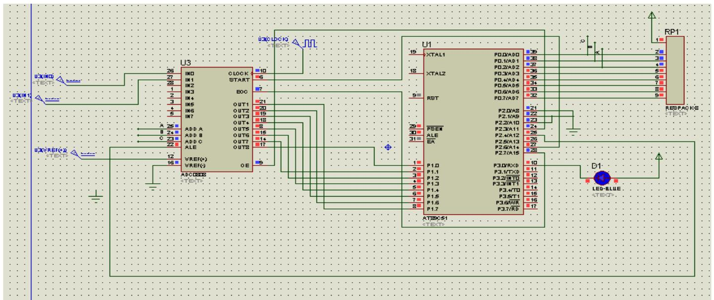
Figure 9. PROTUES simulation for percent differential protection
